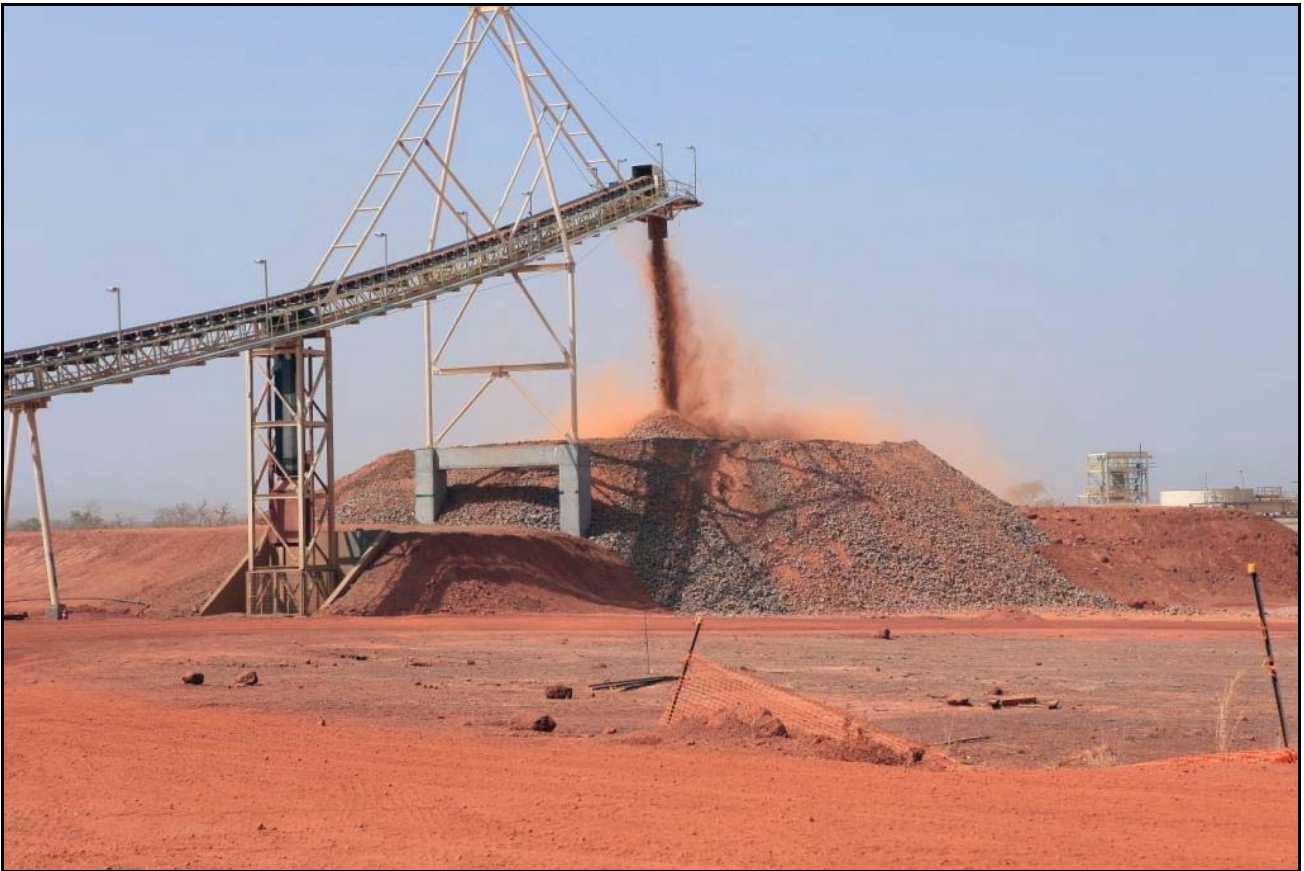
Crushed ore forming the fine ore stockpile
