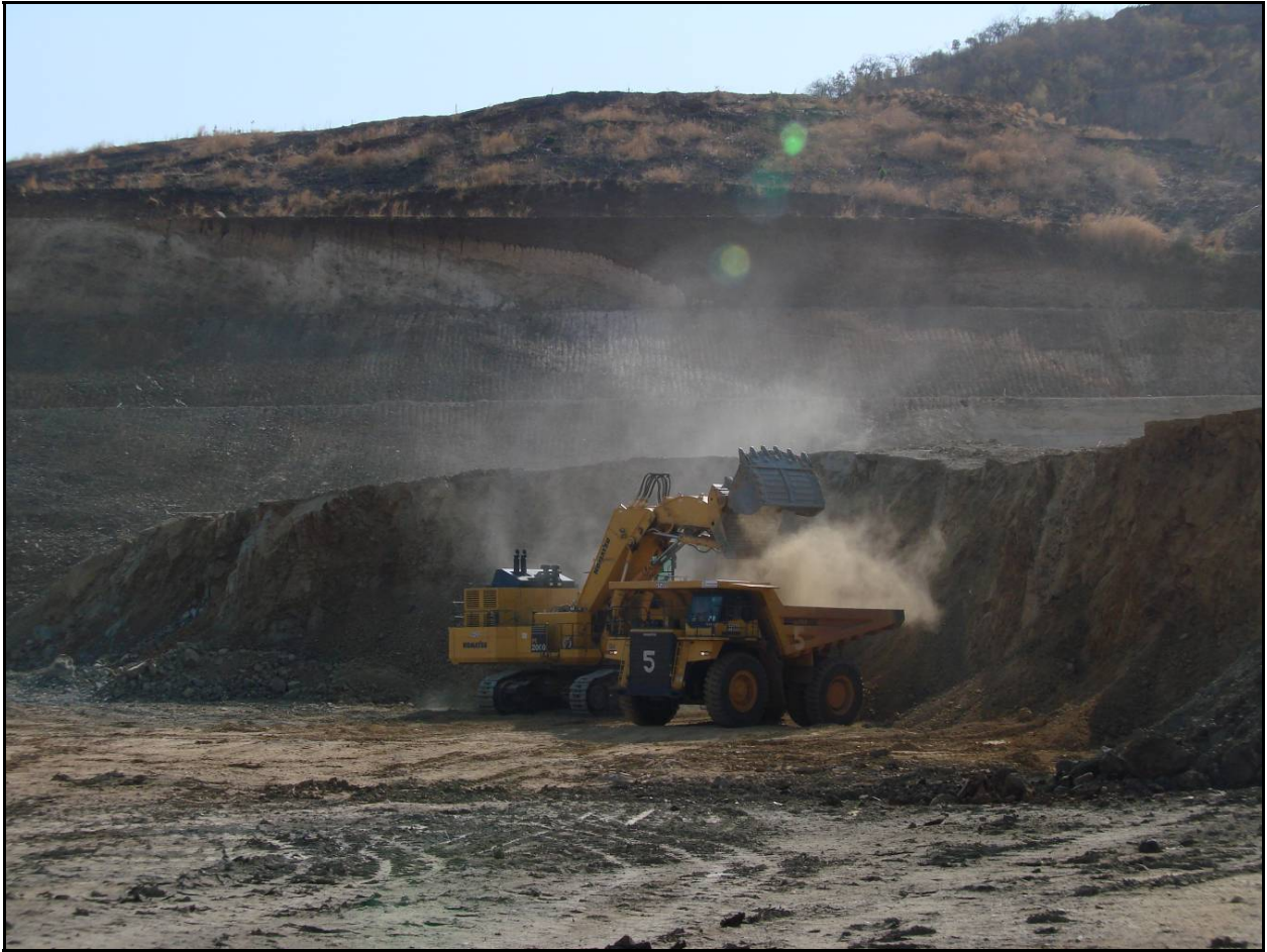
Open pit showing 27 tonne shovel loading 100 tonne capacity truck
