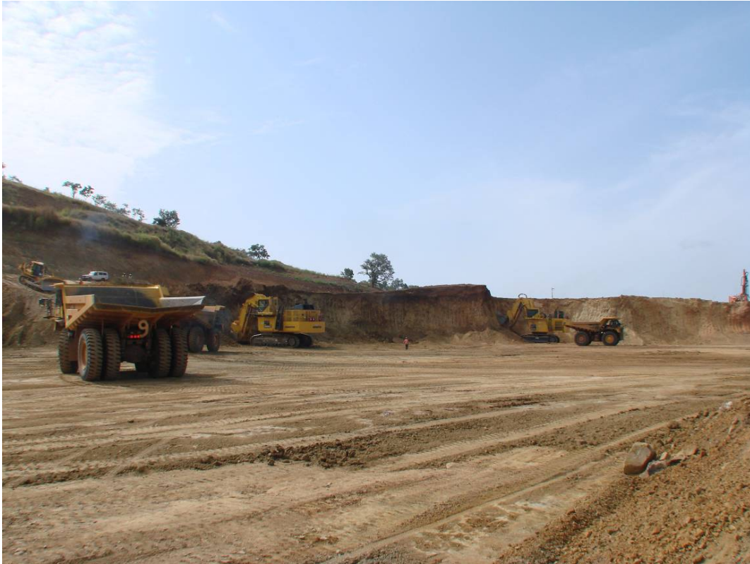
Shovels stripping waste from the 710rl bench of the Sabodala pit in October 2008
