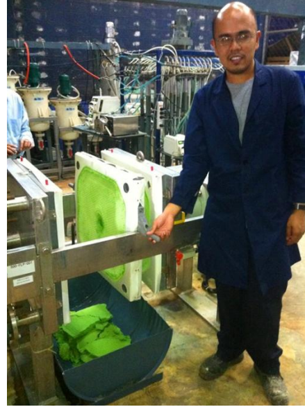
Pilot Plant Metallurgist Vito Andada demonstrates the production of NHP from a filter press at the Agata Nickel Project pilot plant in Intertek Minerals Philippines.
