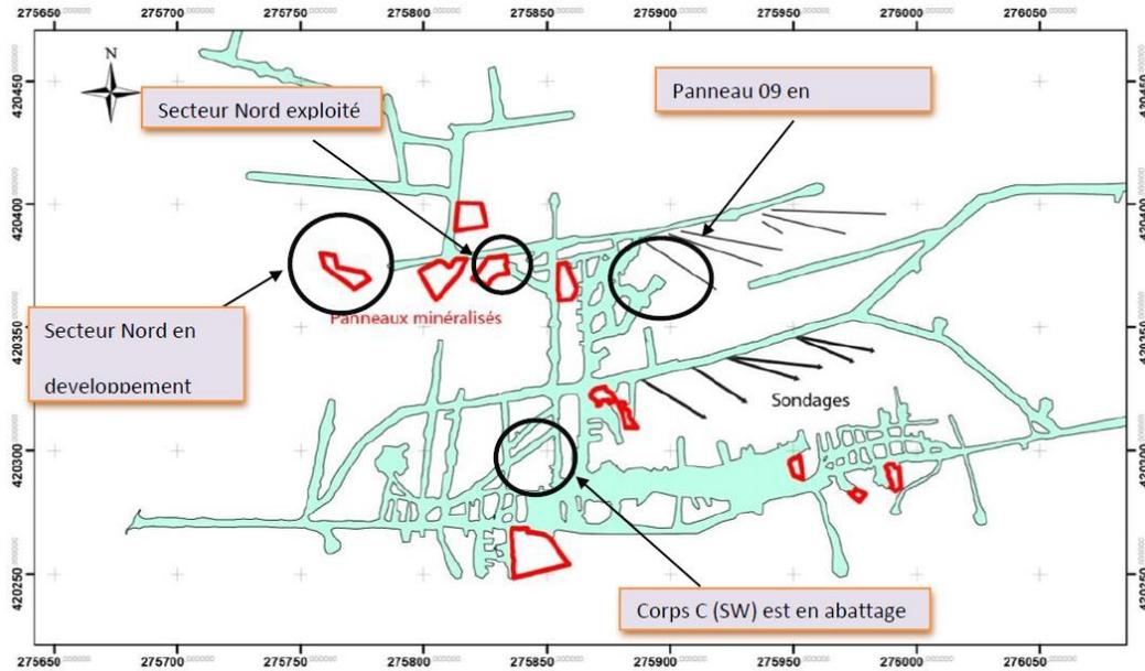
Zgounder Silver Mine / Plan view of the underground workings with sectors being mined & developed at the 2000 Level.
