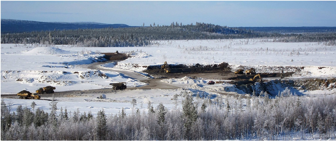
Removal of overburden at the Tapuli section at Kaunisvaara.
