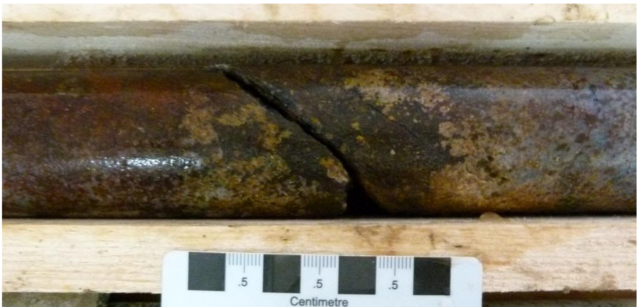
Fig 6 Arrow: coarse pitchblende mineralisation in vein, RK-14-21, 318.5m
