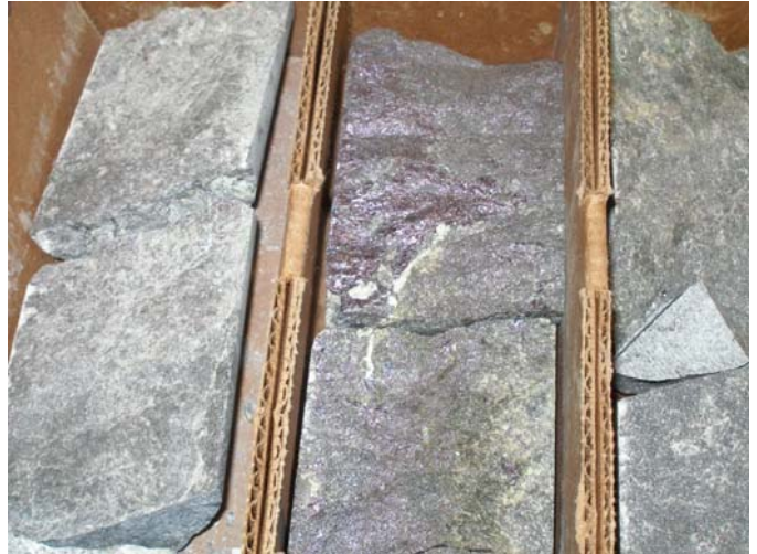
Exhibit 6: Massive bornite in drill core
