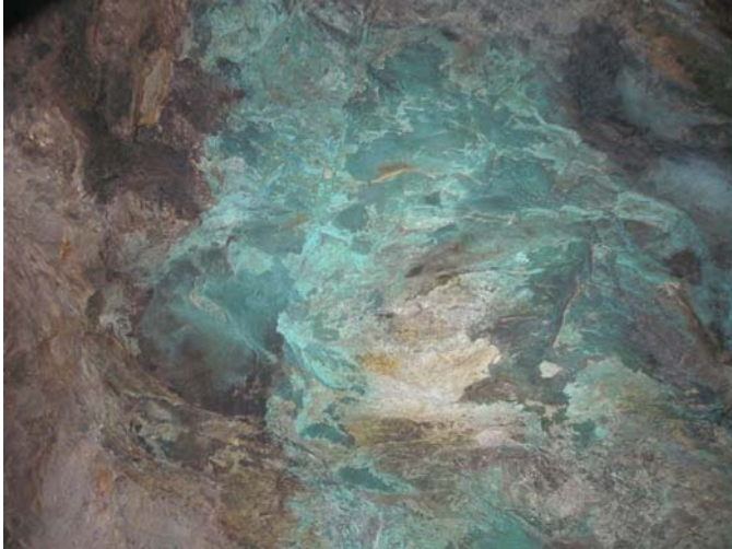
Exhibit 5: Oxidized ore on 6400 Level
