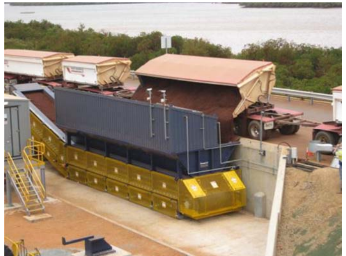
Haulage contractors side tip Spinifex Ridge Iron Ore product into the stockpile facilities at Utah Point, Port Hedland.
