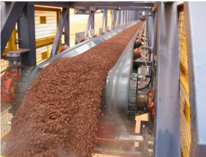
Spinifex Ridge Iron Ore Fines being conveyed to stockpile at Utah Point, Port Hedland.
