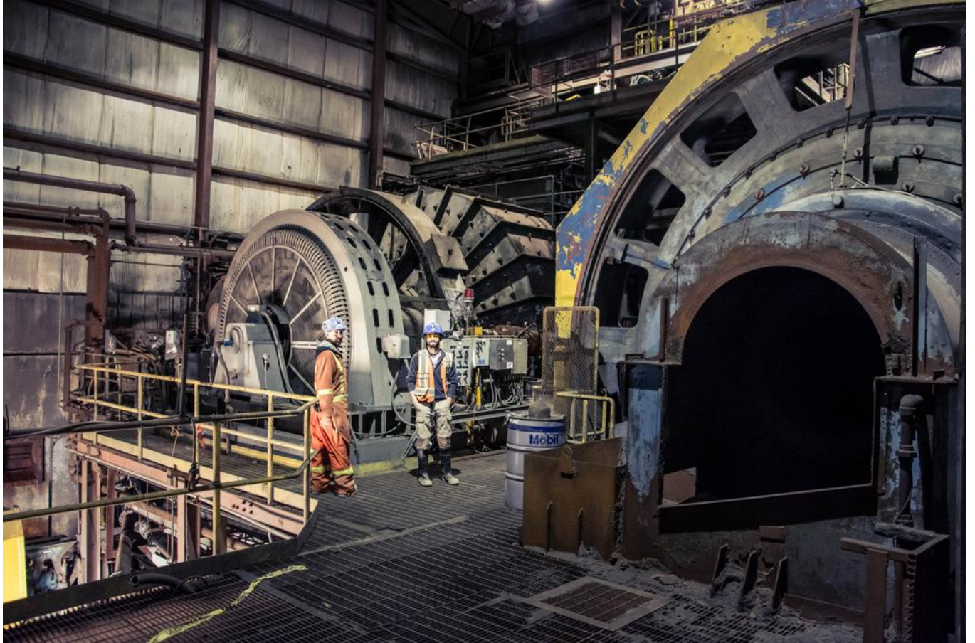
Figure 2: Caribou 3000 tpd SAG mill (in background) scheduled for replacement with new SAG onsite
