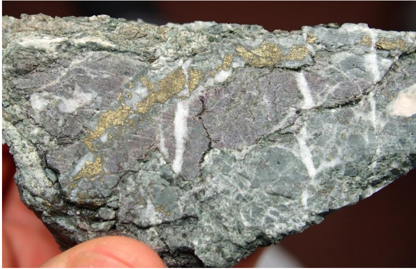
Figure 1. Photo of core from CH-18 @ 511 m (0.8% Cu), showing chalcopyrite veins with a carbonate and kspars stockwork zone in metavolcanics
