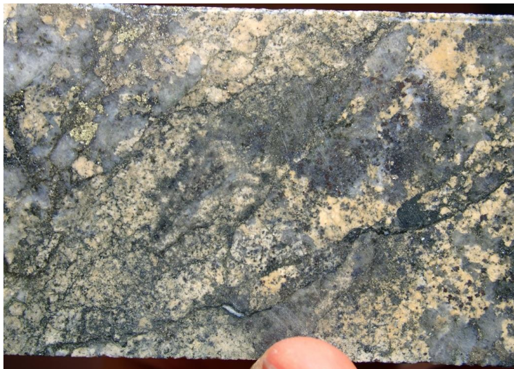
Figure 2. Core running about 119 g/t Ag from CH-28 @ 108 m, showing intense kspars alteration with silica and finely disseminated base-metal sulfides (strong QSP alteration)
