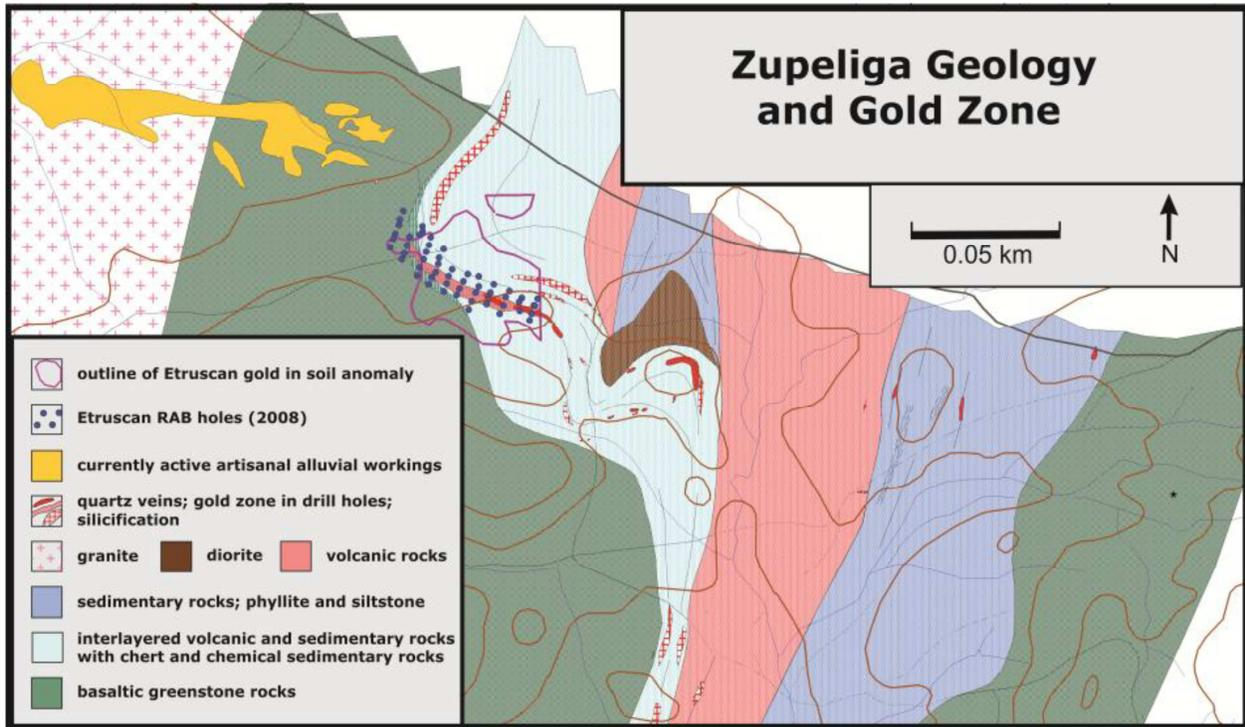
Figure 3. Geologic map of the Zupeliga area showing the location of Etruscan drilling, outline of the Etruscan surface anomaly, and strike extensions of the mineralized zone through regional fold patterns.
