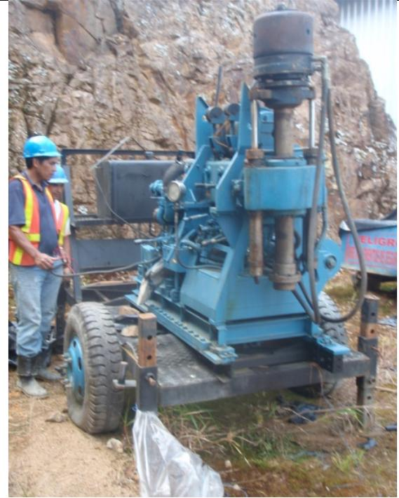
MD-2 man-portable diamond drill for shallow testing IP Chargeability and soil geochemical anomalies
