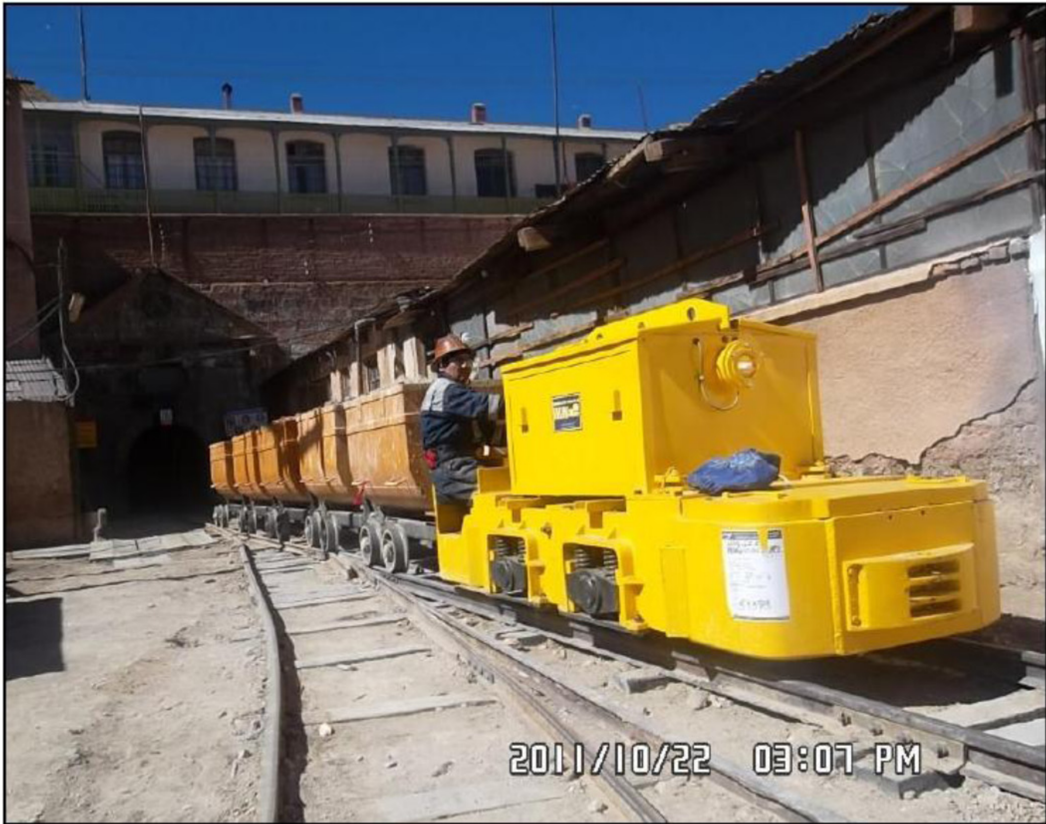
Figure 3: Underground locomotive with 2 ton ore cars exiting the Pulacayo Mine Two larger locomotives with 5 tonne mine cars are expected on site in Q1 2012
