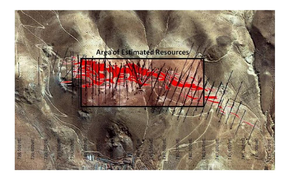
Figure 2. Surface Projection of "Tajo Vein" System showing limits of systematic diamond drilling included in the resource model.
