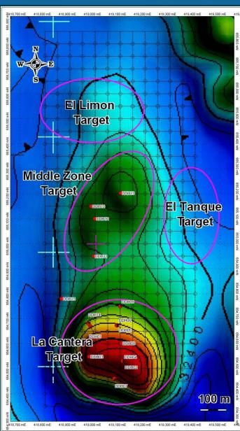
Map showing the location of the geophysical grid over the La Cantera, Middle Zone, El Tanque and El Limon targets. The grid is approximately 1.5 km long and 0.6 km wide. Geophysical lines are spaced 50-m apart.
