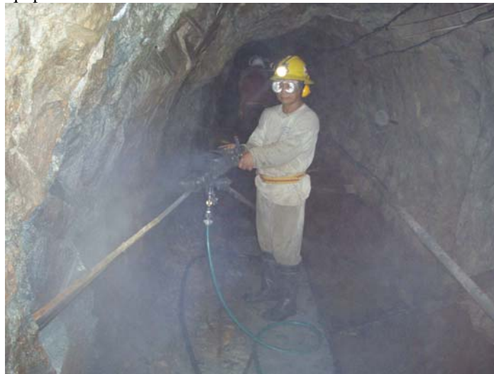
BELOW: The ventilation and alternative egress shaft which is being advanced some 100m ahead and to the east of the “Mafoko Portal” of the decline face. This shaft is being sunk on a gold lode and will provide early trial production when the advancing decline is connected.
