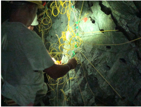
Preparing for the first blast of the planned production-exploration decline to access part of a mineralized zone
