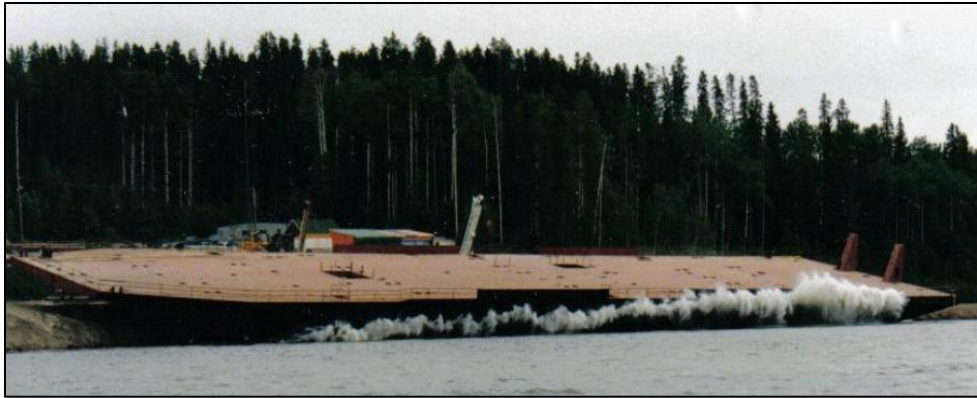
Launch of the MV Williston Transporter, which was built on the shore. Cardero Coal will also complete construction of their tug and barge on the shore.
