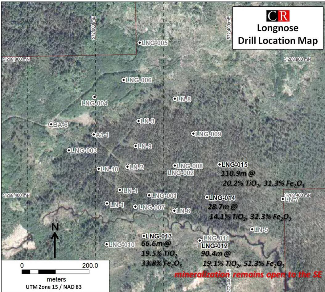
Figure 1: Drillhole locations at the Longnose Ferro-Titanium deposit
