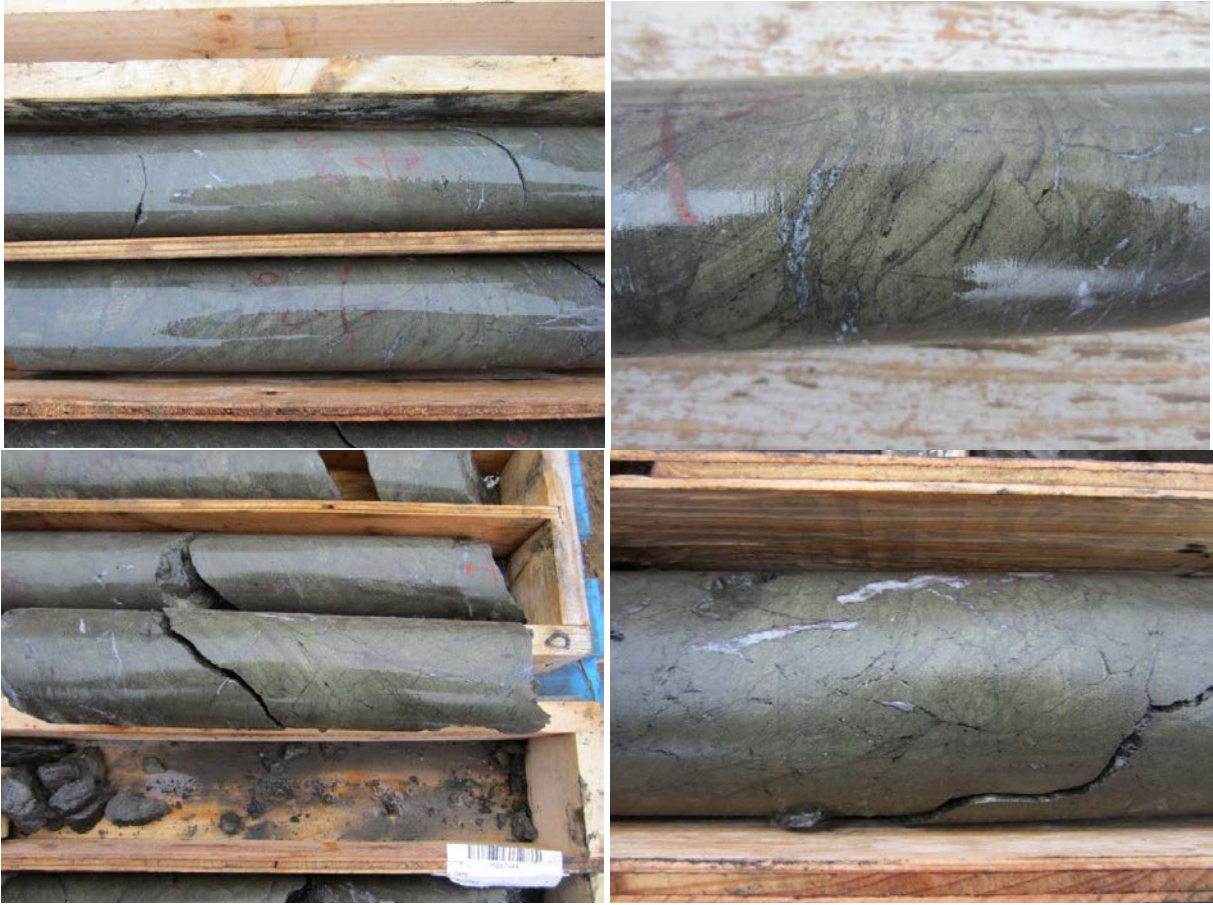
Copper-rich massive sulphides intersected from 137.5m depth in drill hole CD15-14 (HQ-sized diamond drill core; 63.5mm diameter)
