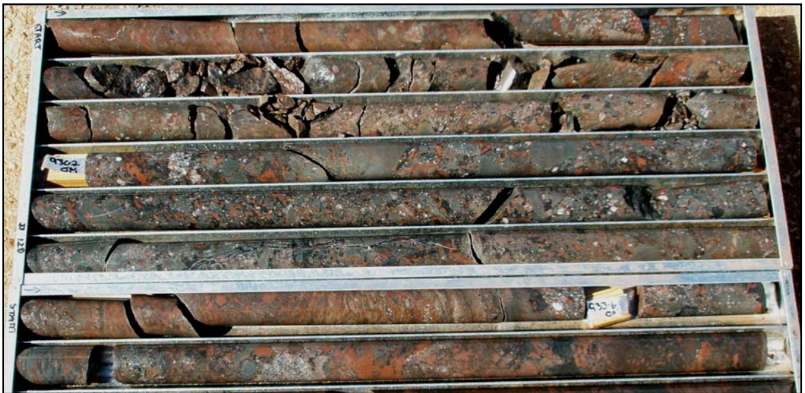
Photo 4: Interpreted heterolithic collapse breccia (Approx downhole depth 930m).
