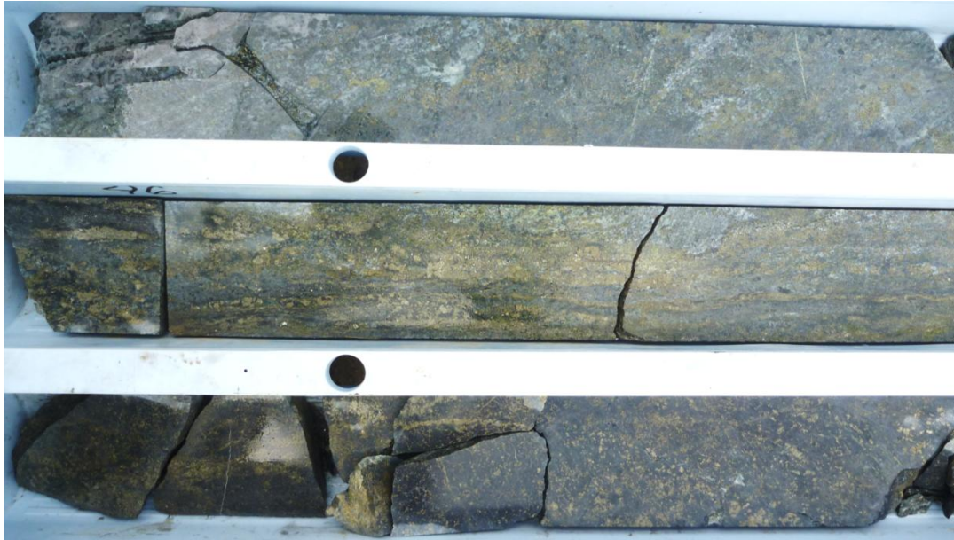
Figure 2 - Mineralised porphyry interval in hole BCPDH00006 45.00m-47.00m downhole direction to the right, 2.00m @ 0.48% Cu, 0.19g/t Au, 1.6g/t Ag; shows steep sheeted py-cpy-mt veins (centre) with surrounding magnetite (bottom) and quartz-magnetite (top) alteration of host granodiorite.
