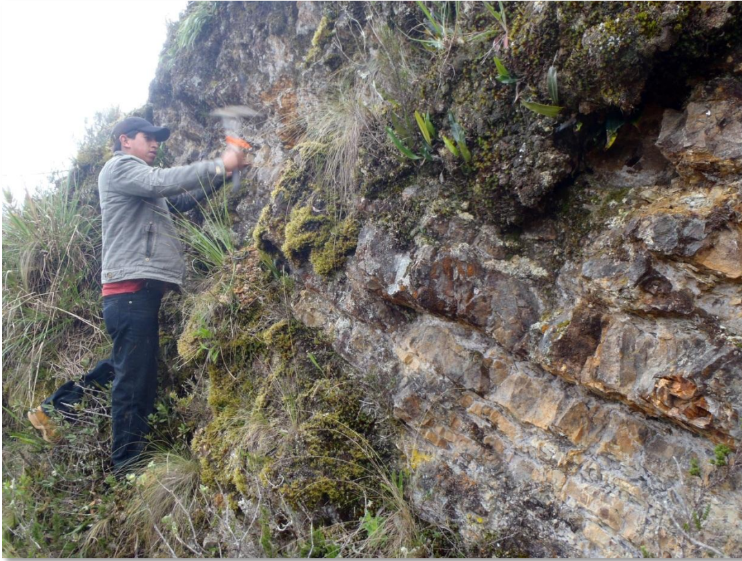
Figure 4: Sampling of gossanous, thin-bedded sandstone-siltstone.
