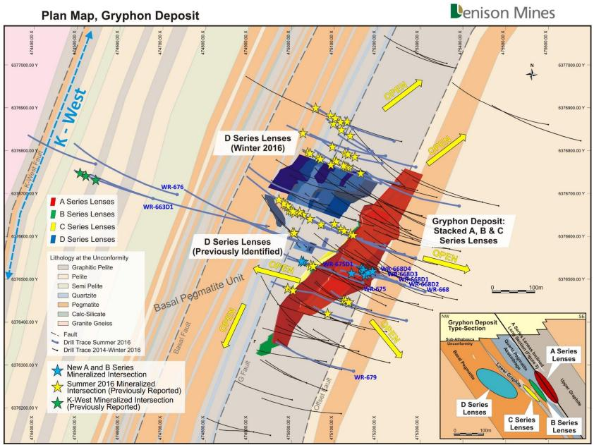
Figure 2: Plan map of the northeast plunging Gryphon mineralized lenses projected up to the simplified basement geology at the sub-Athabasca unconformity. Light blue stars depict the location of new mineralized intersections from the A and B series lenses.
