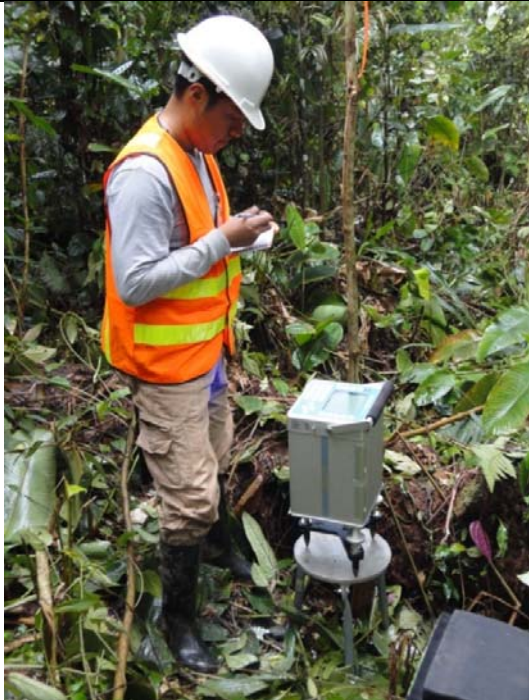
Operator and Scintrex CG-5 gravimeter
