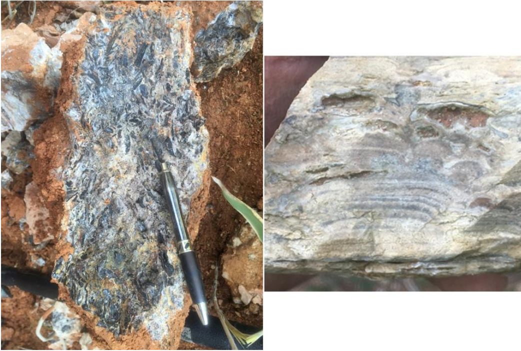
(Figure 2: Vein breccia from Omui mine (left). Fine dark chips of chalcedonic quartz are cemented by late stage sugary white quartz. Siliceous sinter displaying layered fossilized microbial mat near the bottom (right). Field of view is about 4 cm. Such sinter forms in pools at surface as hot spring fluids cool once they emerge from deep in the ground.)
