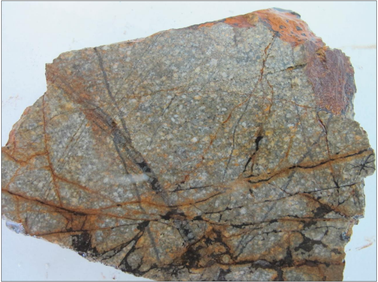
Figure 4: Image of potassic-altered, plagioclase-phyric diorite porphyry from exploration trench DGRCH011 showing quartz-magnetite-chalcopyrite veining cross-cut by later stage pyrite veining (phyllic alteration); 0.43g/t Au, 0.06% Cu; field of view is 14 centimeters.
