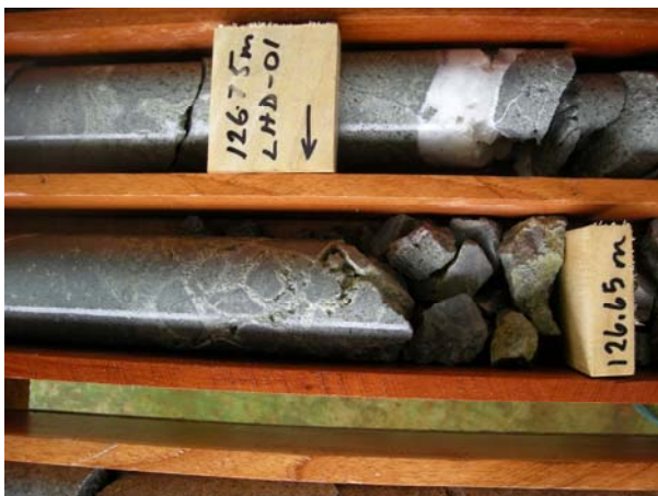
Photo 3 LHD-01 (126.75m) Breccia zone within a sheared and strongly sericite-pyrite altered andesitic sequence.
