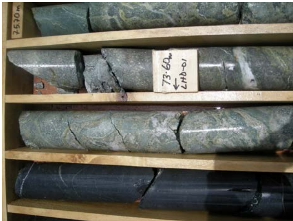
Photo 1 LHD-01 (73.60m) Pseudo-breccia zones in intensely sheared andesitic sequences. Advancing alteration fronts (intense quartz-carbonate-chlorite-pyrite) produces pseudo-breccia textures.
