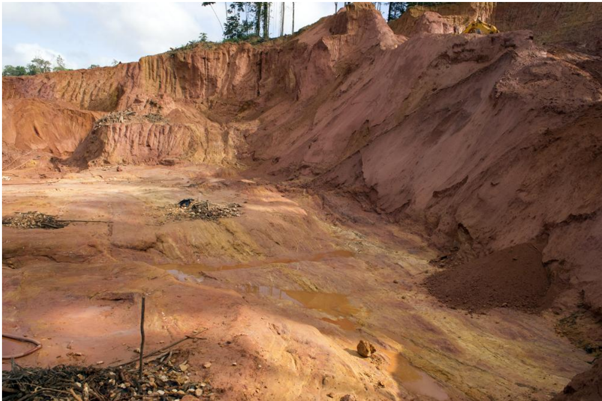
Figure 2: View northwest along strike of the mineralization (pale orange and yellow) at Jons Pit. The first diamond drill hole is collared on the bench where the excavator arm can be seen (top right).
