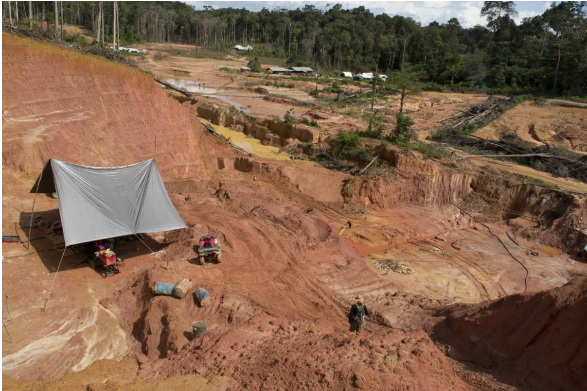
Figure 1: Drill rig collared 40 metres northeast from mineralization at Jons Pit Prospect. Note large scale of artisanal workings centred on deformed quartz veins and veinlets with limonitic quartz-iron carbonate selvage.
