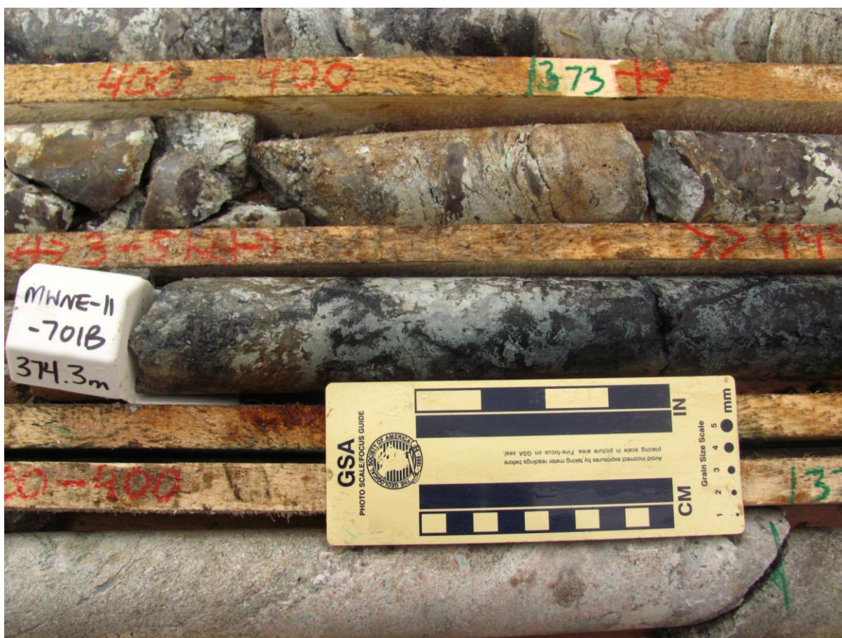
Figure 7. Alteration at Far East. Upper photo: extensive hematite alteration in drill hole MWNE-11-704. Lower photo: hematite and complex clay (chlorite and illite) alteration in drill hole MWNE-11-701B.
