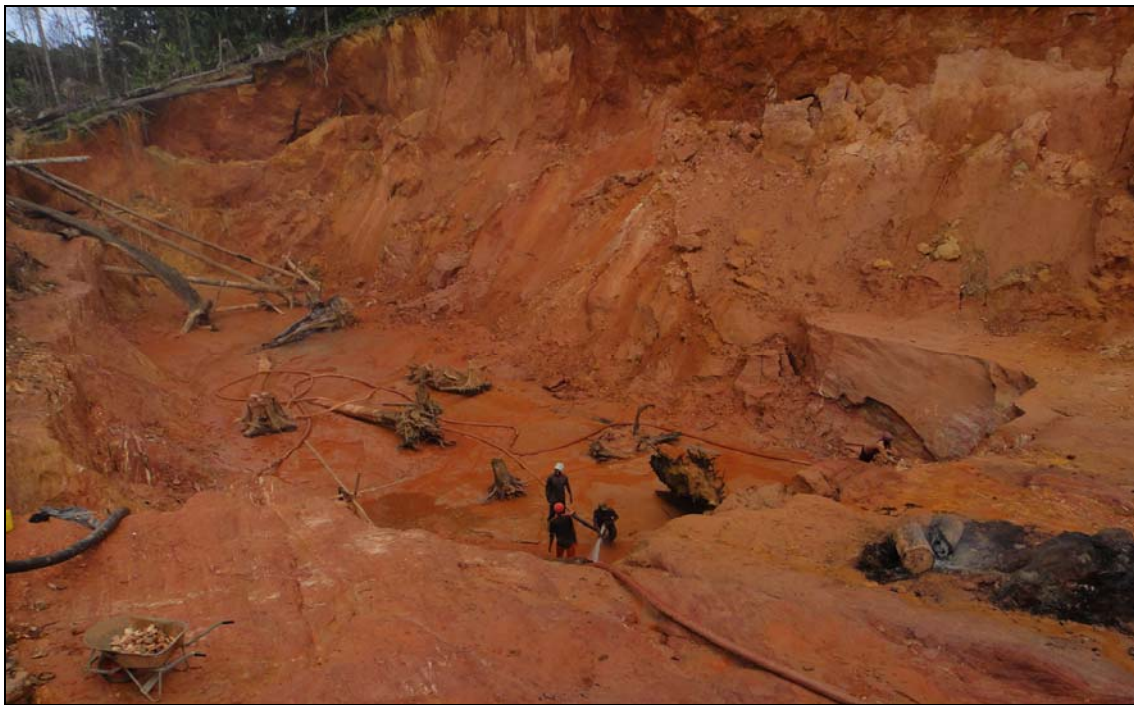
Figure 5: Photograph at Jons Pit prospect showing artisanal miners hydraulically excavating limonitic saprolite which represents the upper supergene altered part of a shear zone. Gold is recovered using simple sluice boxes.
