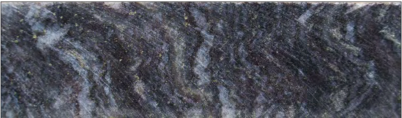
Figure 4: SKD001, 107.3 m: Schist. Dark grey-green, fine-grained, micaceous matrix, moderately silica-chlorite altered with moderate disseminated, fine- to medium-grained pyrite. Crosscut by sub-parallel and deformed quartz veinlets composed of blue-grey, fine-grained, translucent quartz. Crosscut by rare pinkish carbonate veins. From a 1.0 m interval which assayed 4.69 g/t gold (107.0 to 108.0 m).
