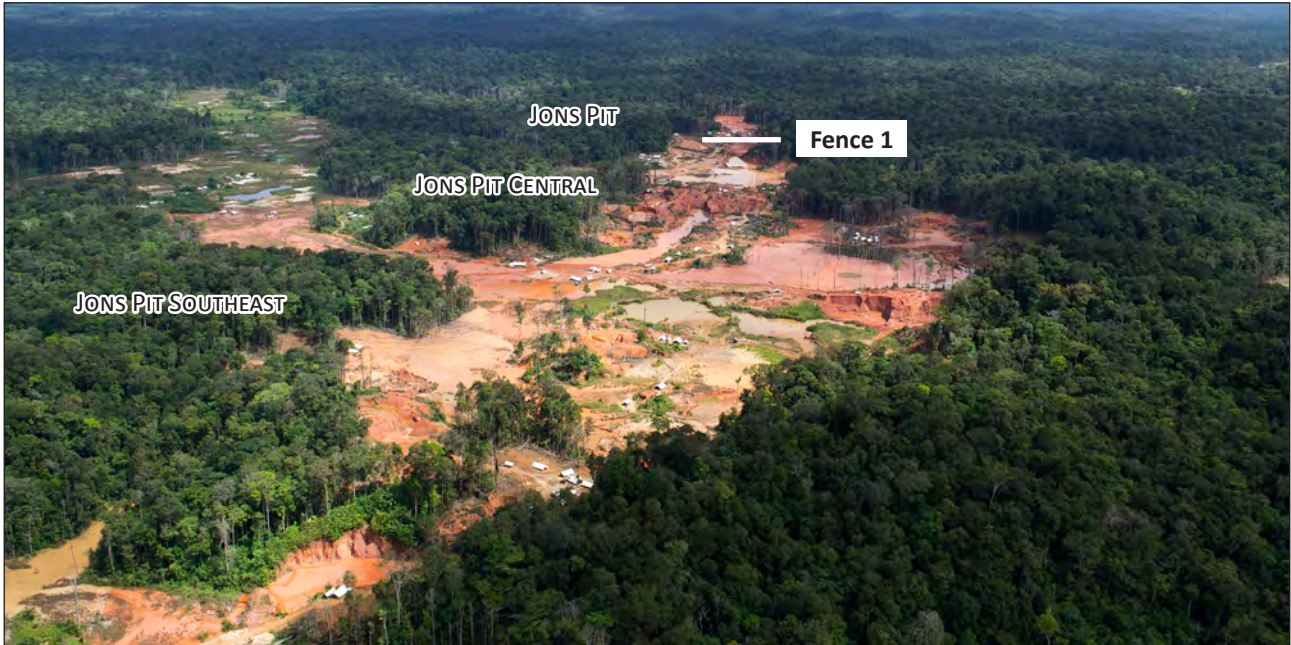
Figure 3: View west-northwest along strike of the 1.6 km long Jons Pit Prospect, Sela Creek. Note Fence 1 is located at the far west-northwestern end of a series of artisanal workings exploiting saprolitic parts of a shear
