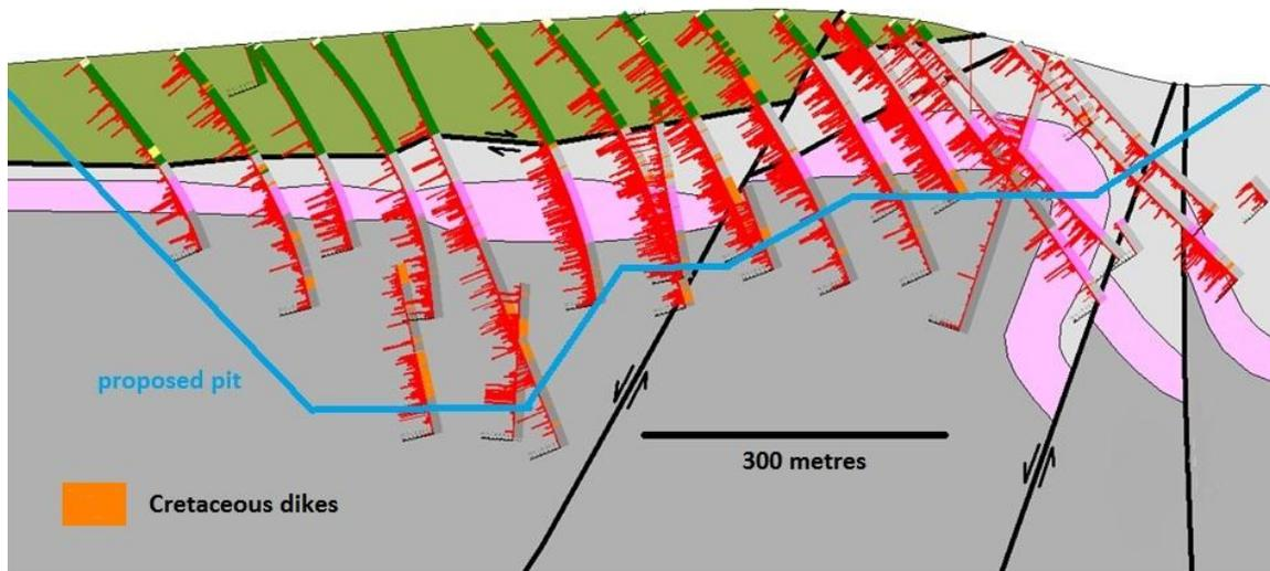
Figure 2: Cross section 428925E of the Money Knob gold deposit looking west. Note the association of the strongest mineralization with the volcanic section (pink unit) and dikes (orange).
