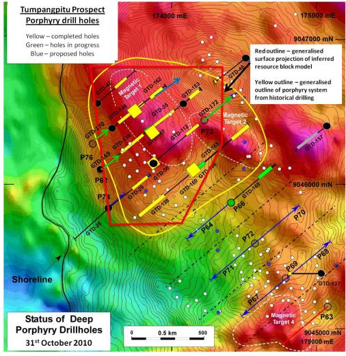
**Drill status plan:** Collars of oxide holes shown in white and blue. Deep drill traces shown in black, and proposed in blue. Those holes that have been completed are shown in yellow bars, and those in progress shown in green bars.
