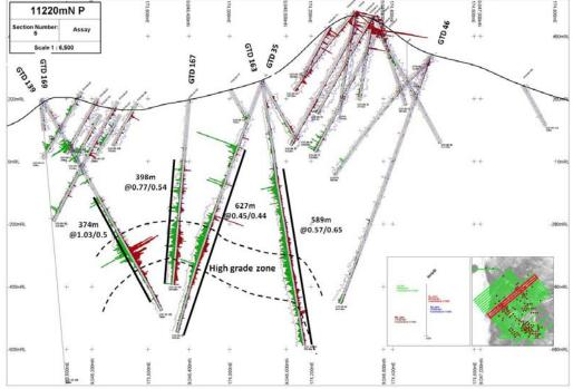
**Cross Section** through central part of currently known porphyry system showing hole GTD-167 relative to holes 139, 35, and 163.
