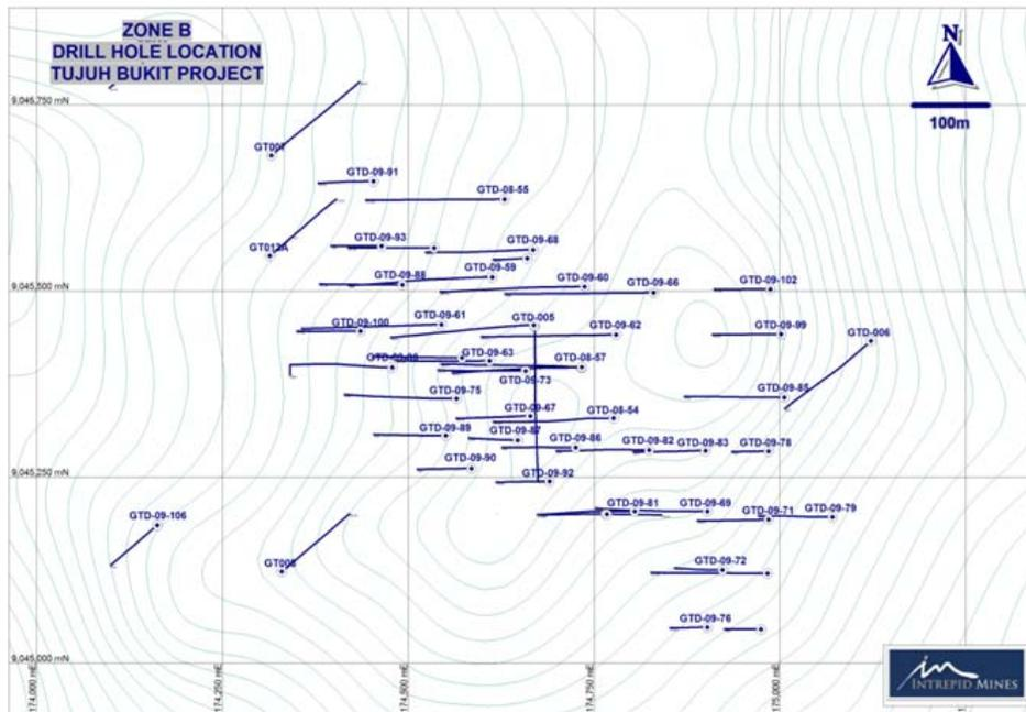
*Diagram (UTM grid lines are at 250m intervals) showing the location of drill holes within Zone B. The holes have been drilled primarily to the west (Intrepid-IMN drilling), with a few to the northeast and southwest (Placer drilling). Hole dips are mostly -60 degrees, though they vary from -45 to -80 degrees (see section below).*
