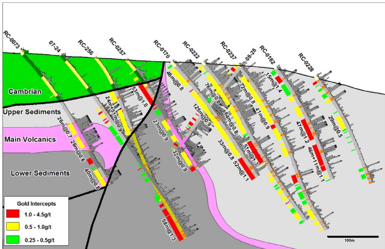
Figure 1: Section 429525E illustrating intercepts and the continuity of the mineralization in the Sunshine Zone.
