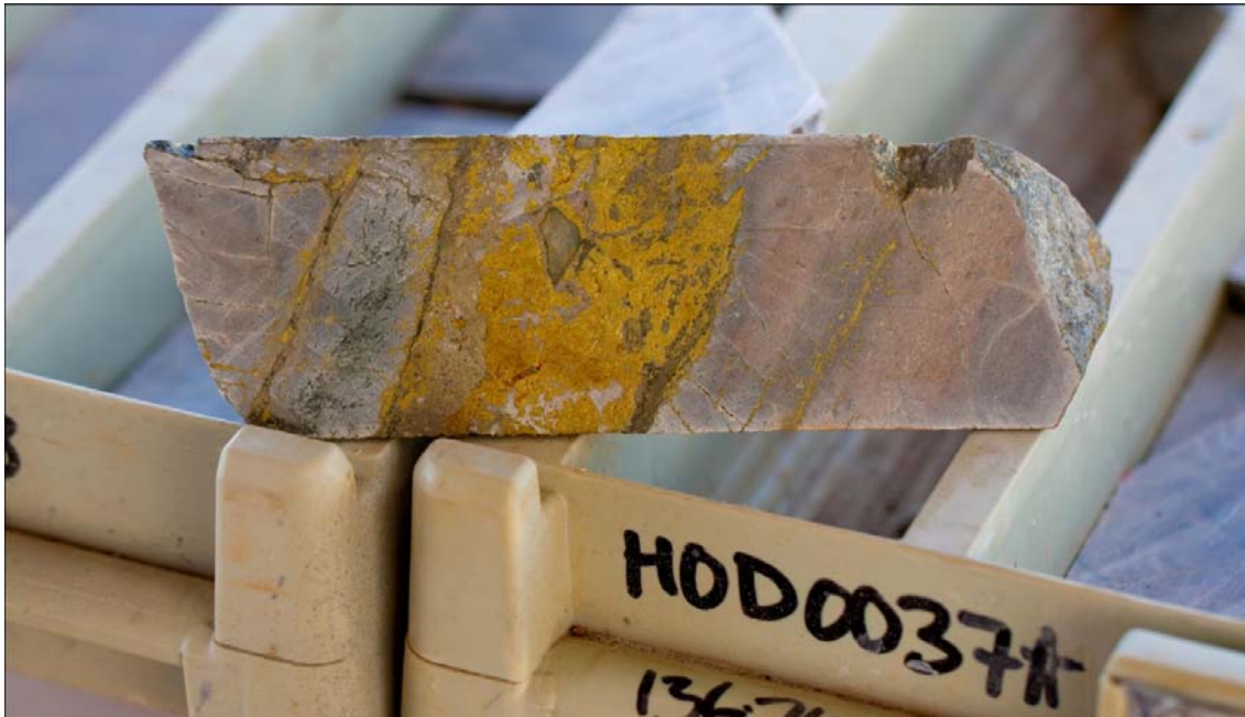
Figure 6: HOD0037A - Massive chalcopyrite veining with feldspar altered muscovite schist
