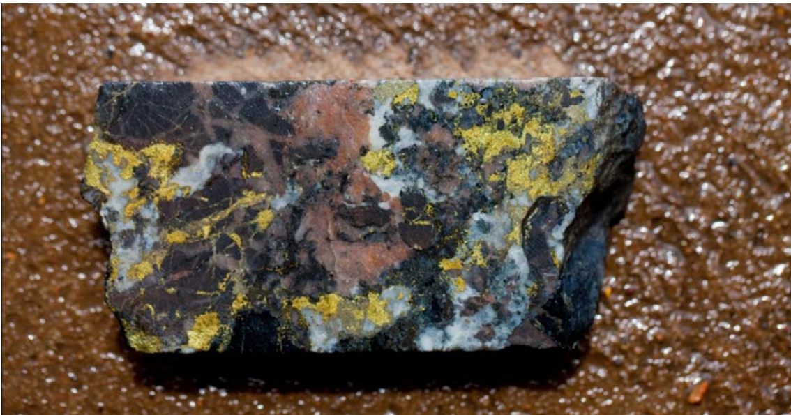
Figure 5: HOD0038 - Brecciated amphibolite. Breccia matrix consists of calcite, chalcopyrite, quartz and hematite stained feldspar
