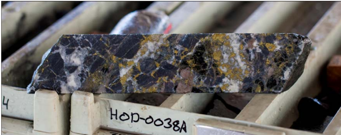
Figure 8: HOD0038A - Brecciated amphibolite. Breccia matrix consists of calcite, chalcopyrite, quartz and hematite stained feldspar
