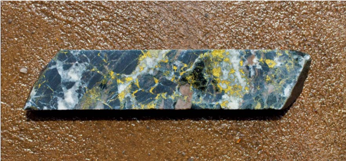
Figure 4: HOD0038 - Brecciated amphibolite. Breccia matrix consists of calcite, chalcopyrite, quartz and hematite stained feldspar
