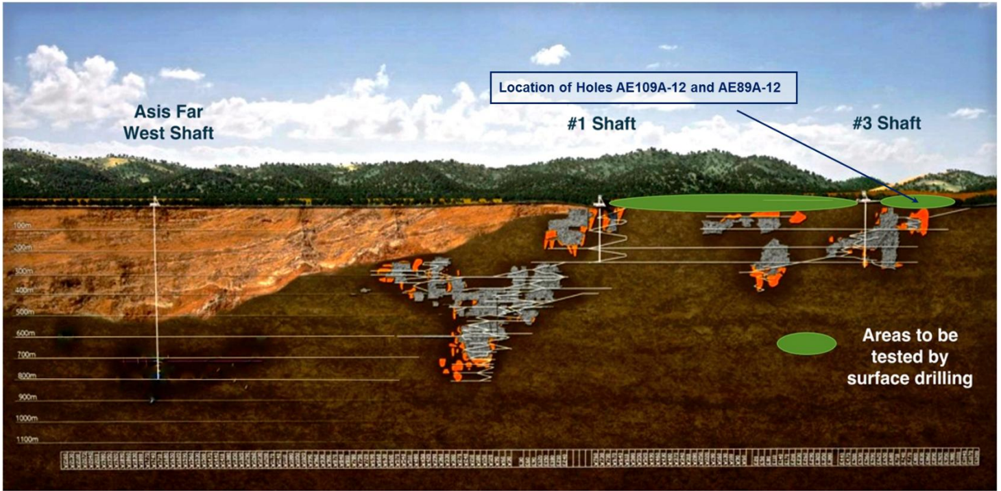
Figure 2: Longitudinal Section of the Kombat Mine Identifying Areas Drilled
