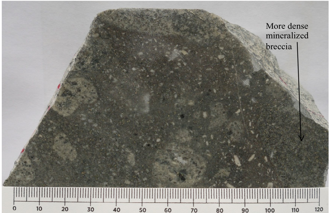
Photo. Mineralized porphyry in hole F82, with multiphase breccia (0.55% Cu, 0.5g/t Au at depth 177 metres)
