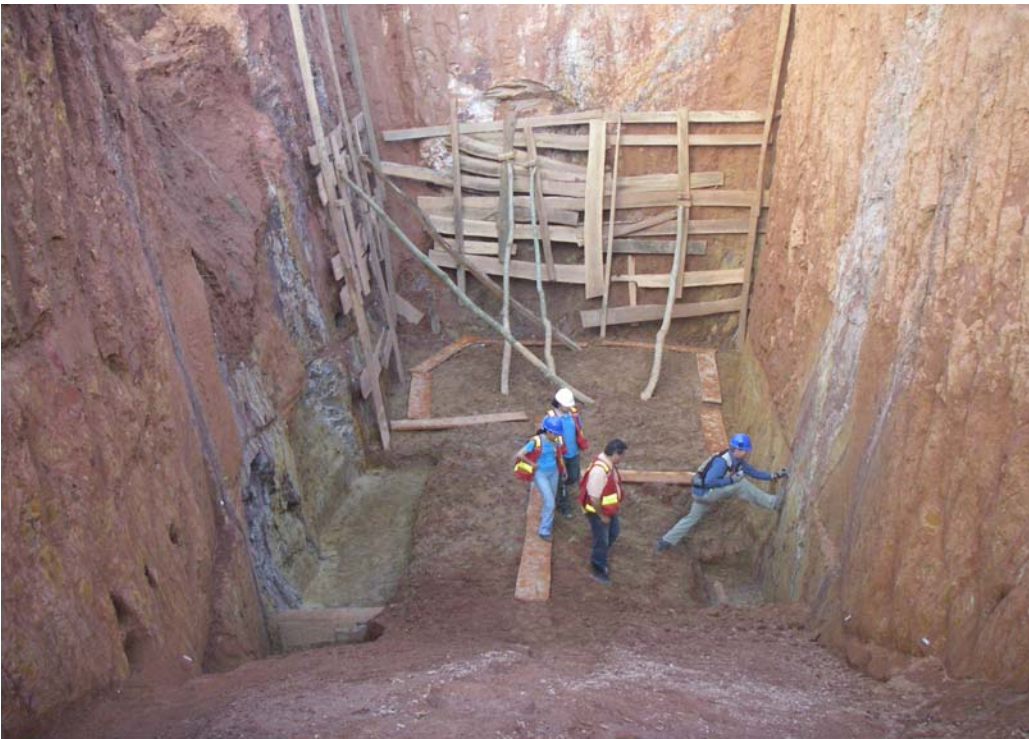
Picture 2: Trench 3. Project geologists examine a gold shoot running 10 gpt Au across 0.5 metres. Notice the extension of the shoot in both sides of the wall.
