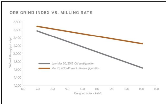
*Note: the higher the ore grind index, the harder the ore being processed in the SAG mills.*
