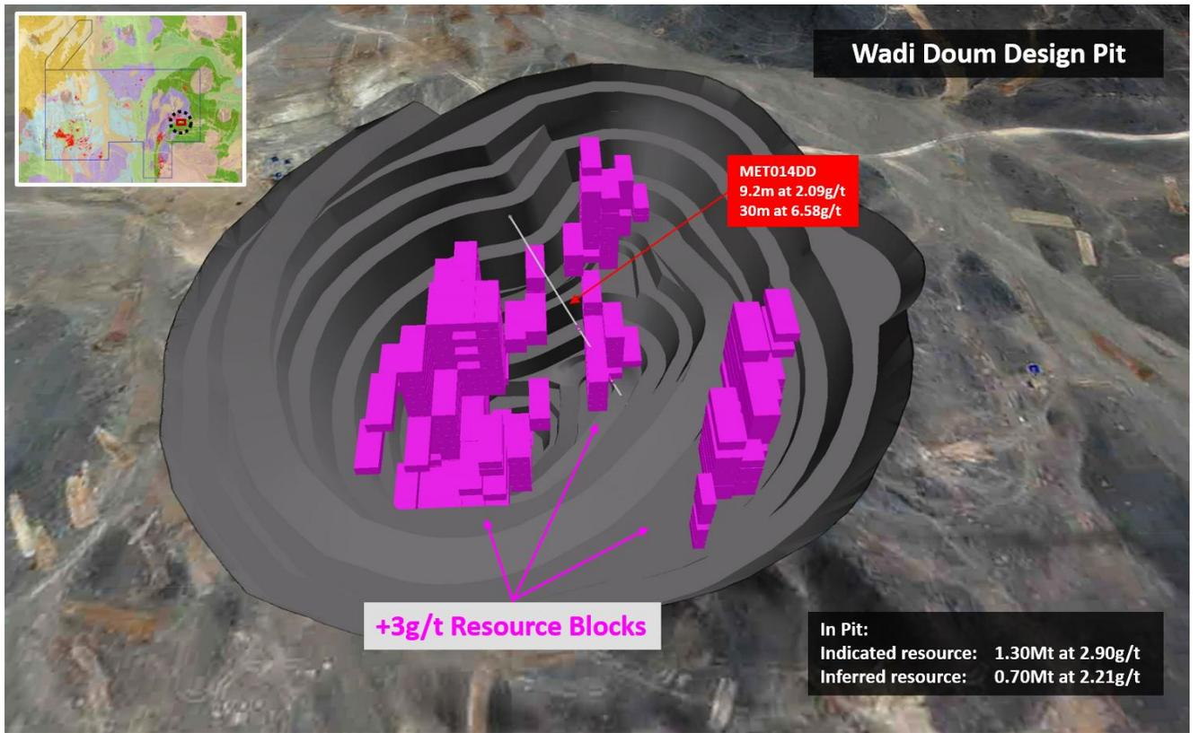
**Figure 2: View of Wadi Doum showing pit design, MET014DD drill hole trace and +3g/t resource blocks**
