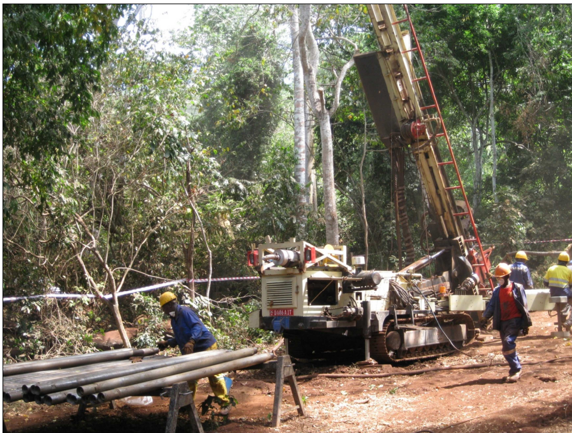
Photo 2: Track mounted RC drill team and local laborers at hole PAWRC040.
