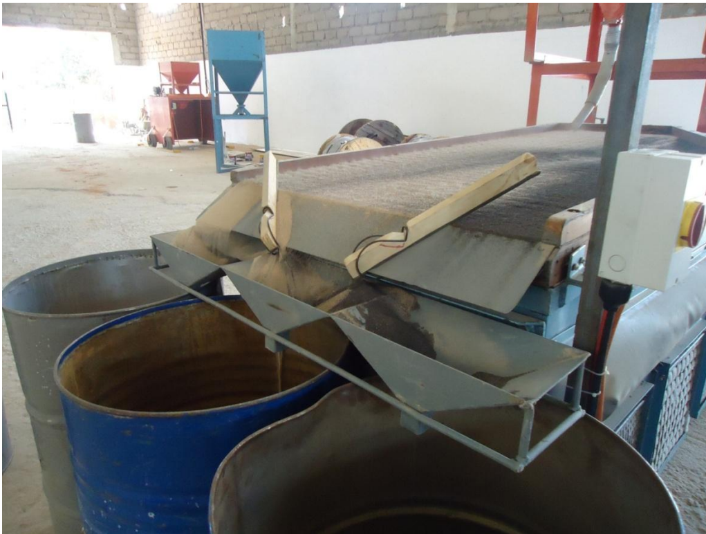
Figure 6 – Table Producing Secondary Tantalum Concentrate
