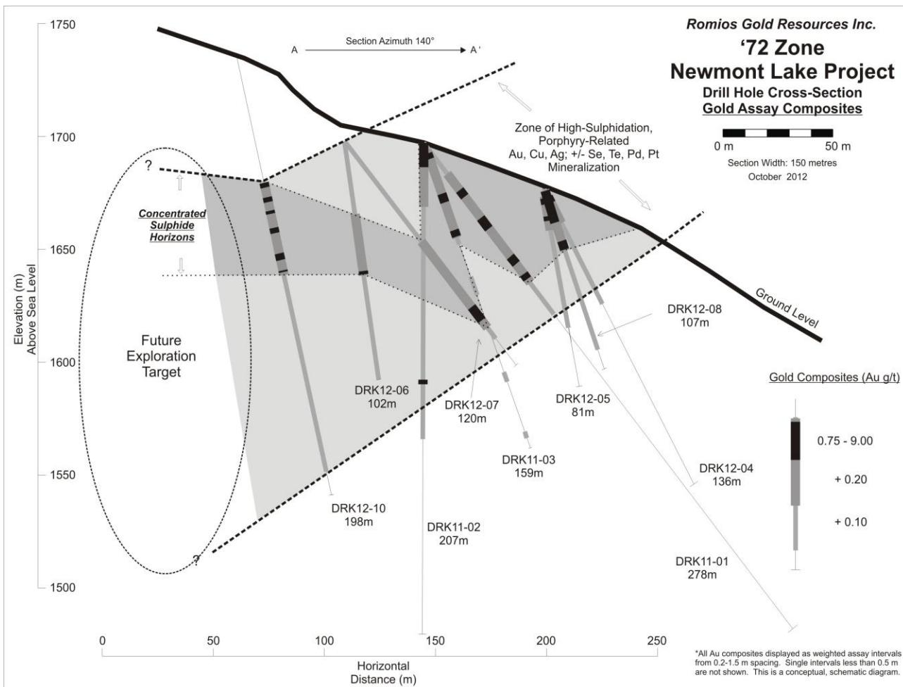
\*All Au composites displayed as weighted assay intervals from 0.2-1.5 m spacing. Single intervals less than 0.5 m are not shown. This is a conceptual, schematic diagram.
