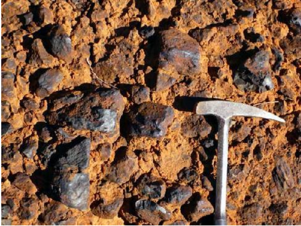
Figure 5 - Typical surface appearance of indurated detrital ironstone composed of poorly sorted, framework supported, angular clasts of hematitic-goethitic ironstone and BIF.
