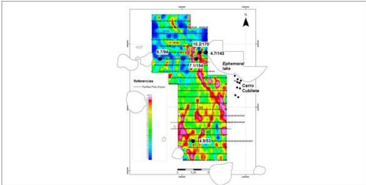
*Figure 1. Corina lag sample grid showing Au anomalies and I.P. image. Anomalous lag values are shown as large black circles with values indicated as ppm Au/ppm Ag. Small black dots are drill-holes at Cerro Cubilete*
