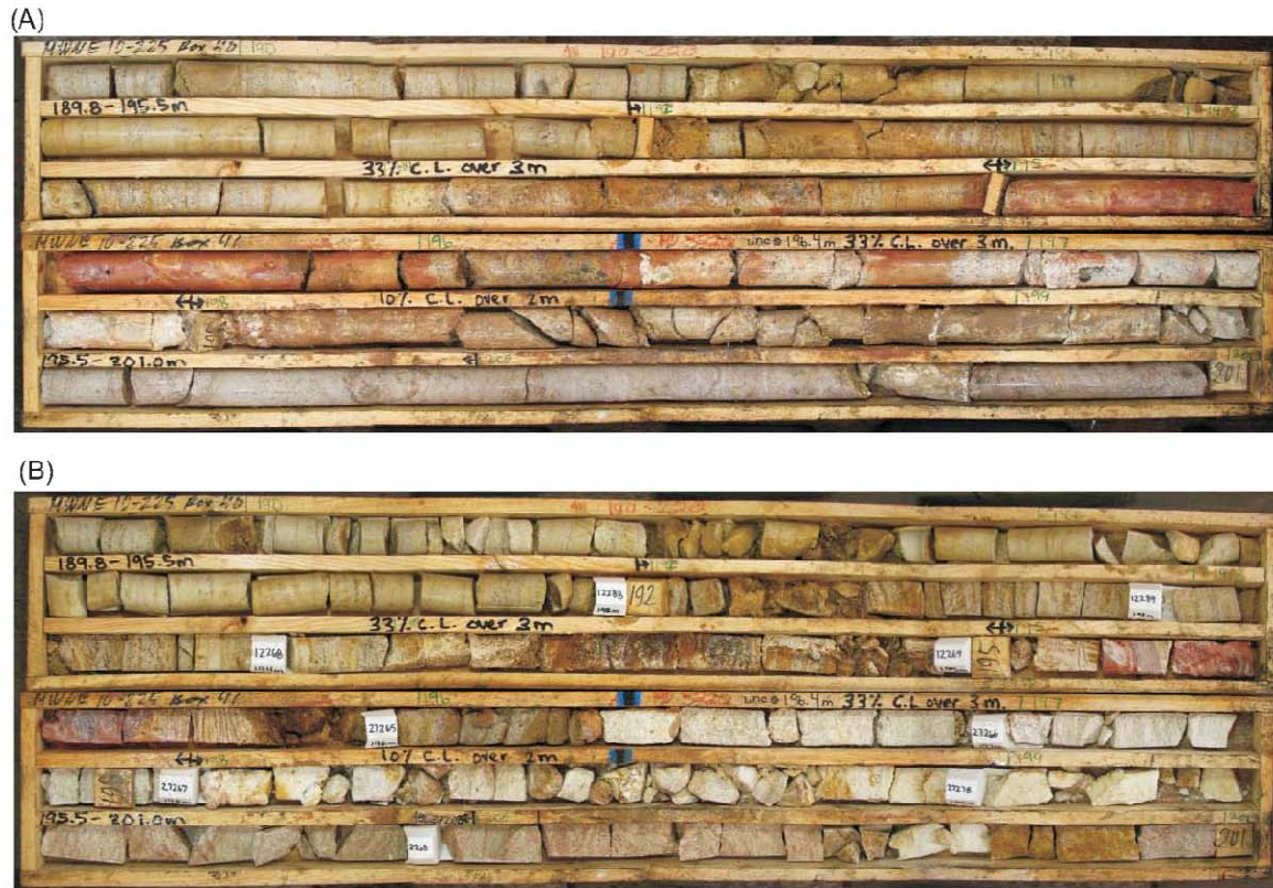
Figure 1: Drill core photograph of MWNE-10-225 from 189.8 to 201 m, showing clay alteration before split sampling (A) and after split sampling (B).
