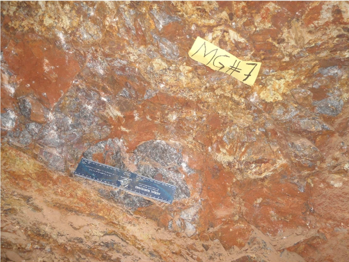
Figures 1-3: Well defined quartz veining and sheared metavolcanic rocks hosting high grade gold exploited by artisanal miners on the Tembo Project
