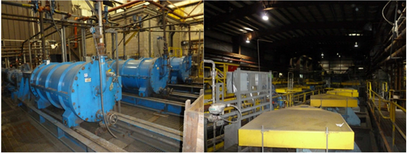
Figure 1: IsaMills (left), part of the grinding circuit at the Caribou Mill complex in New Brunswick, and flotation circuit (right)
