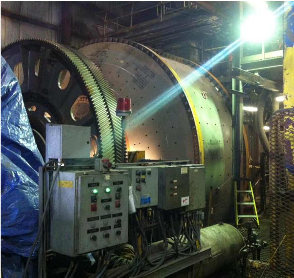
Figure 1: Newly installed 3,000-tonne-per-day SAG mill at Caribou Mine
